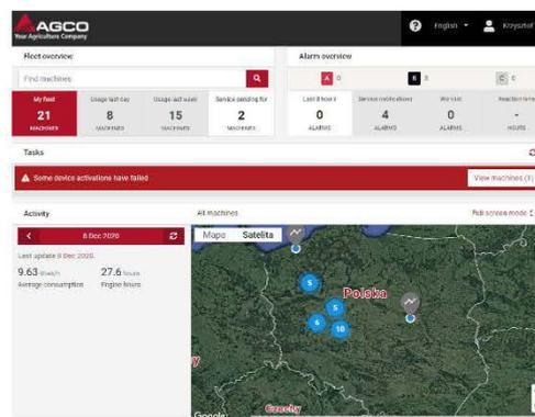
Fig. 4. Telematics website main screen used by authorized technical service of agricultural machines (source: own study based on [15])
