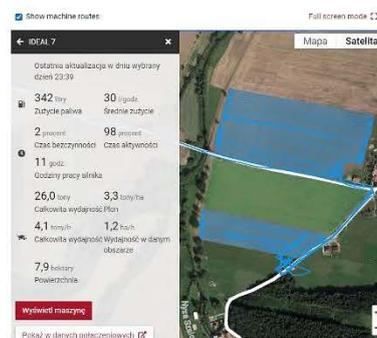
Fig. 2. Preview of work parameters and drive trails in AGCO Connect app
