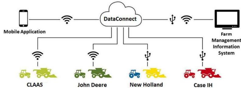
Fig. 3. Data transfer scheme for the DataConnect system (source: own study based on [17])
