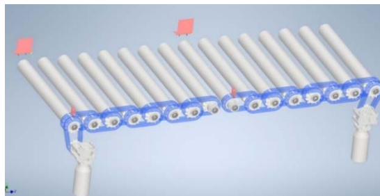
Fig. 3. View of conveyor drive system
