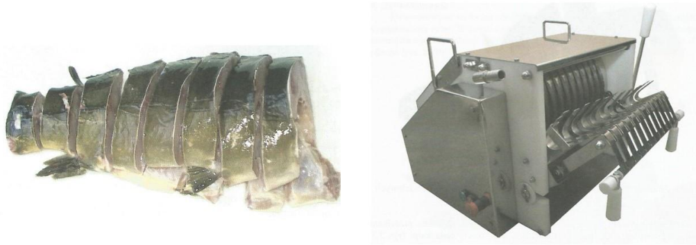
Fig. 3. Carcass of carp cut into darnes, and a machine (prototype) for darne-cutting
