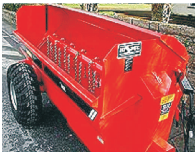
Rys. 7. Rozrzucaacz obornika z bocznym adapterem firmy Hi Spec [7] Fig. 7. Manure spreader with side adapter produced by Hi Spec Company [7]
