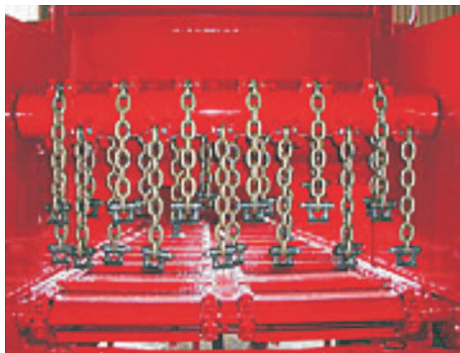
Rys. 5. Rozrzucaacz obornika z adapterem bijakowym firmy Unia Group [6] Fig. 5. Manure spreader with beater adapter produced by firm Unia Group [6]
