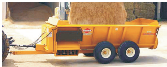
Rys. 6. Rozrzucaacz obornika z bocznym adapterem firmy Kuhn [5] Fig. 6. Manure spreader with side adapter of firm Kuhn [5]
