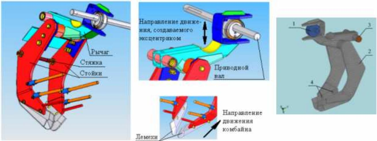
Fig. 1. Beet harvester lifter point constructive scheme and its simplified model
