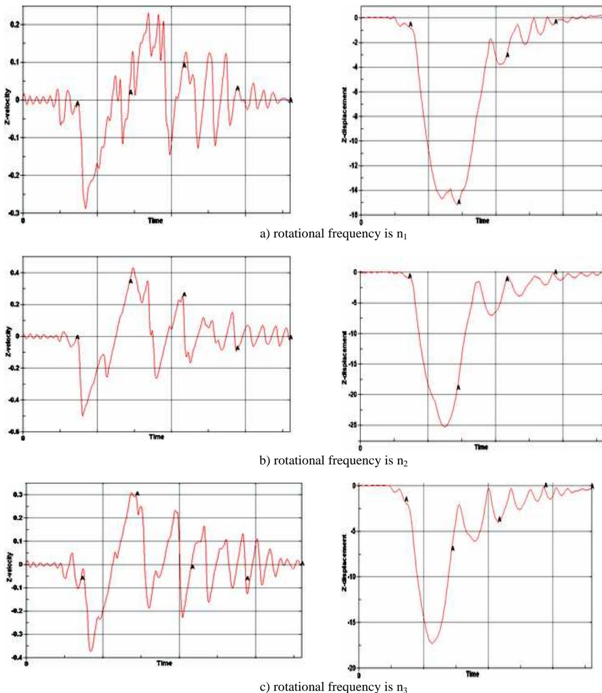
Fig. 6. Nodes displacements and velocities plots of the beetroot at different angular velocities
