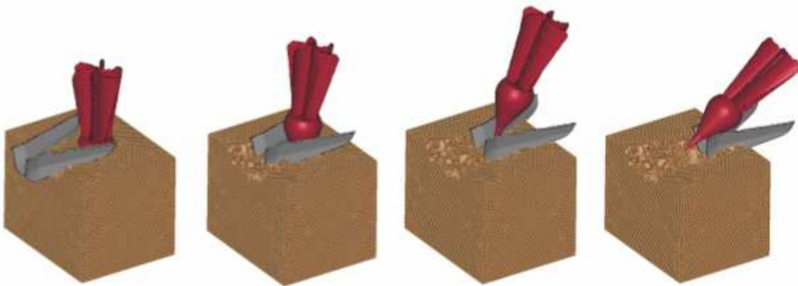
Fig. 3. Beetroot digging out process
