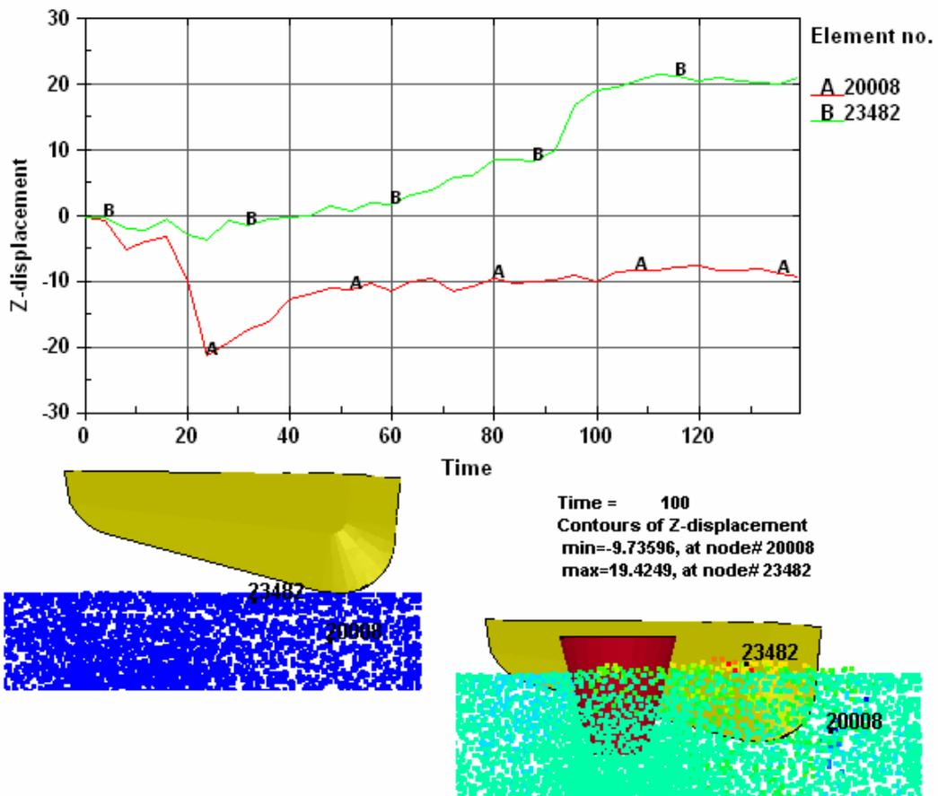
Fig. 5. Relative soil particles displacement due to lifter point movement
