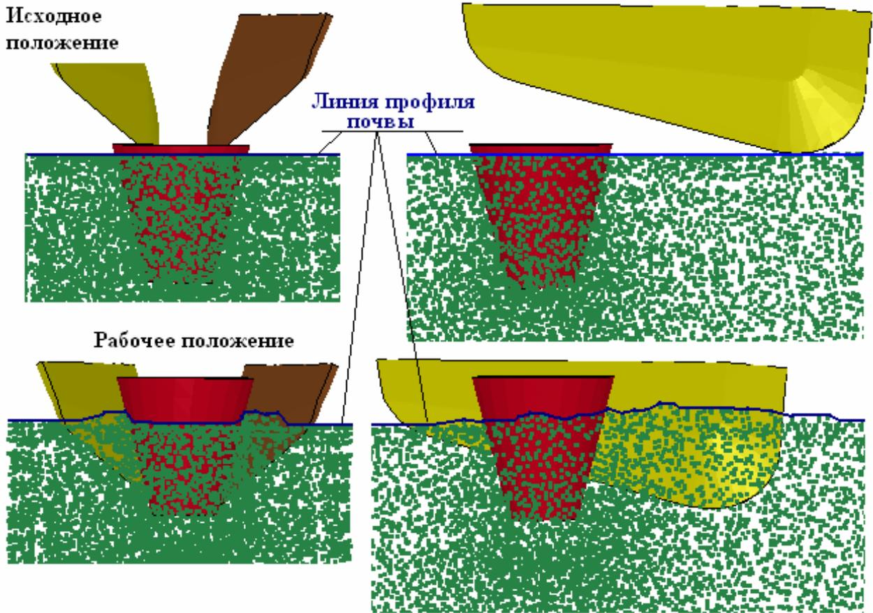
Fig. 4. Soil surface profile changing during lifter point movement
