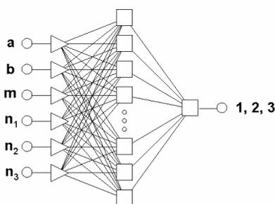
Fig. 3. Structure of developed *MLP* type neural network
