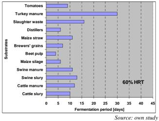
*Rys.* 4. *Time to reach* 60% *of HRT for the tested substrates*
