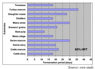
Fig. 6. Time to reach 90% of HRT for the tested substrates
