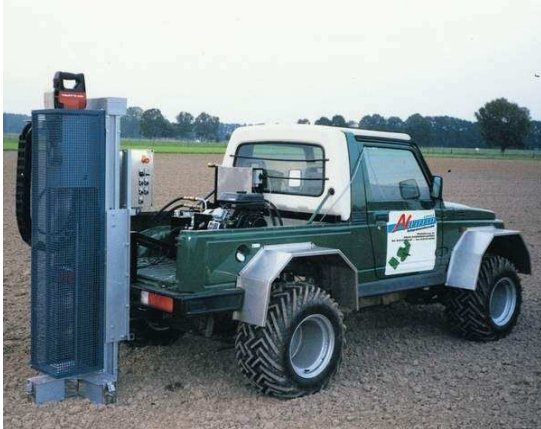
Fig. 1. Vehicles for soil sampling [Agro Technology]
