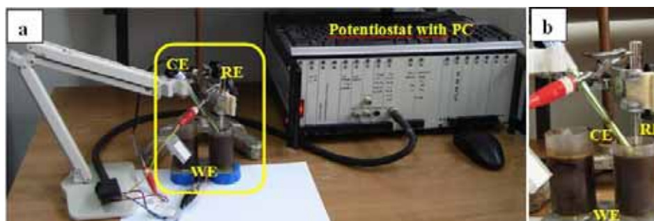
Fig. 1. Set up for potentiodynamic measurements of AISI 304L (EN 1.4307) in animal slurry (a), zoom of the electrochemical cell with counter (CE), reference (RE) and working (WE) electrodes (b)
