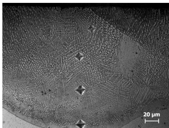
Fig. 8. Microstructure of laser boronized layer
