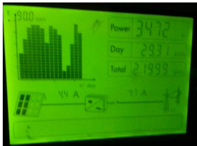
Fig. 1. Monitoring and control panel of the studied solar system
