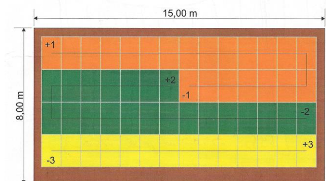
Fig. 2. Schematic layout of groups of solar photovoltaic panels
