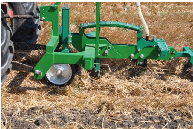
Fig. 2. Model of working section for strip till during field tests
