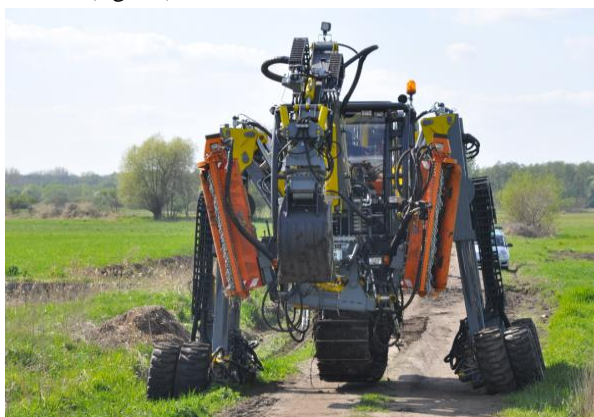
Fig. 22. The movement of the multi-purpose device on a ground road by means of the side wheels
