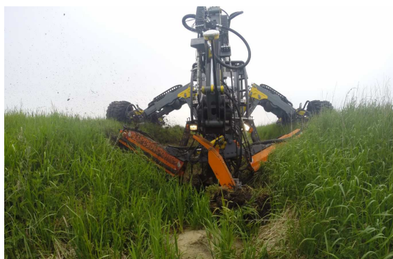
Fig. 8. Watercourse desilting drainage while the cutting plants on slopes
