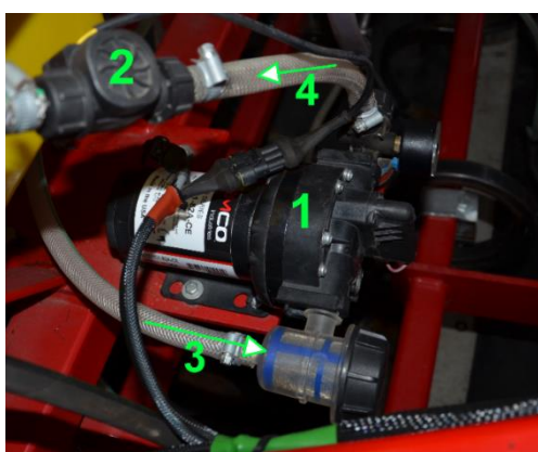
Fig. 2. The pump and components of the control system: 1– membrane pump; 2– flow-meter; 3– the suction pipe; 4– a discharge pipe
