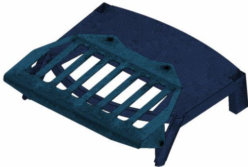
Fig. 6. The finite element model of FOPS
