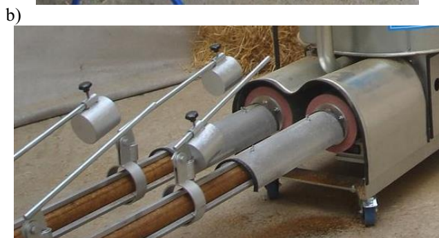
Fig. 3. Stabilizing tracks with different systems of rail pressure: a) with a spring-based system of rail pressure connected to a Pol-lux briquette press [17], b) by Asket, with a lever system of rail pressure [15]
