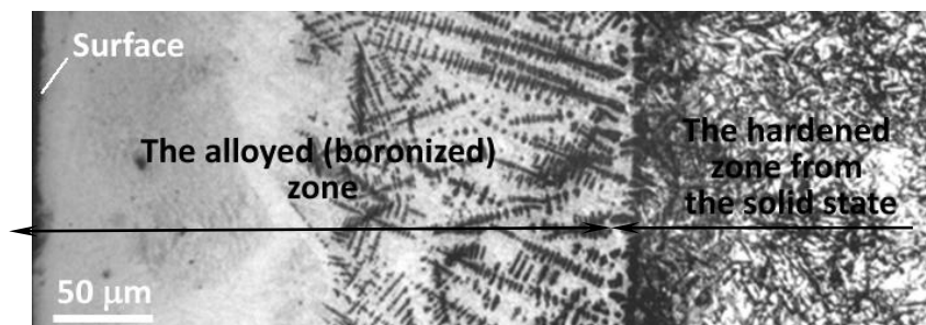
Fig. 1. The cross-section of the surface layer of high carbon alloy steel after laser boronizing. Etched with nitride acid solution. Magnification 500x
