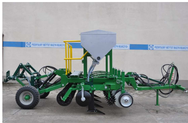
Fig. 1. Unit for Strip-Till and deep application of large fertilizer granules (first working module of research model)
