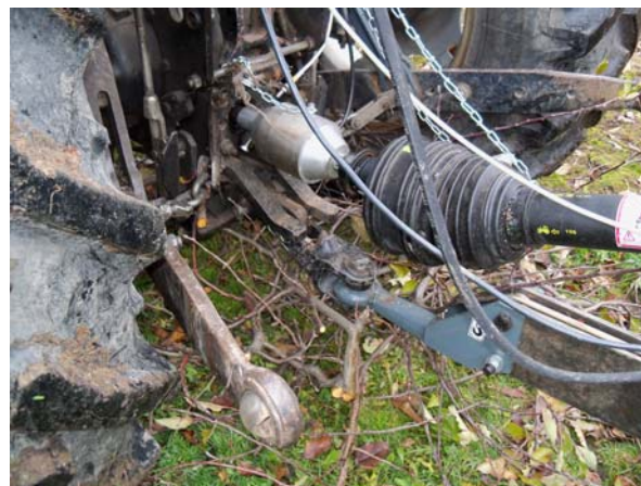
Fig. 2. The MiR 20 torque meter during baler model tests
