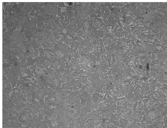
Fig. 2. Microstructure of SSAB BORON B27 steel after austenitising at temperatures: 880°C – A, 900°C – B, 920°C – C and 950°C – D, quenching in water and low tempering at a temperature of 200°C·h -1
