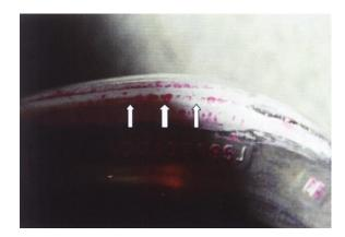
Fig. 9. So called striped cracks in deformed suspension arm detected by penetrant method [7] *Rys. 9. Tak zwane pęknięcia pasemkowe ramienia zawie*-
