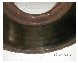
Fig. 3. View of the abrasive worn surface of an exploited automotive brake drum [7]
