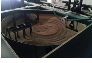
Fig. 2. The "rotating bowl" unit: a) scheme [5]: 1 - transmission, 2 - engine, 3 - running rail, 4 - bowl, 5 - holder of the sample, 6 - supporting frame, 7 - roller: 8 - frame of the bowl, 9 - main frame, b) view [6]
