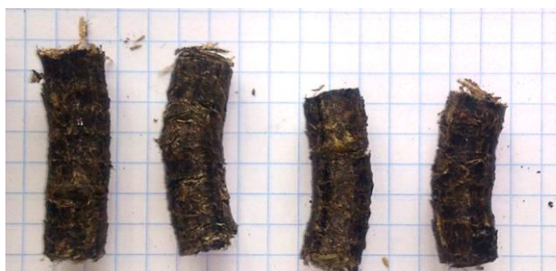
Fig. 6. View of the granulate from a mixture of straw and hard coal with a 15% addition of a potato pulp, obtained at a temperature of 70°C
