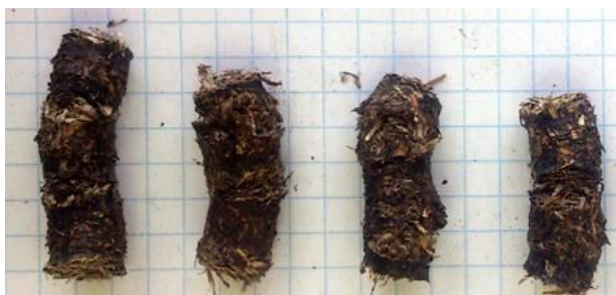
Fig. 5. View of the granulate from a mixture of straw and hard coal with a 20% addition of a potato pulp, obtained at a temperature of 70°C
