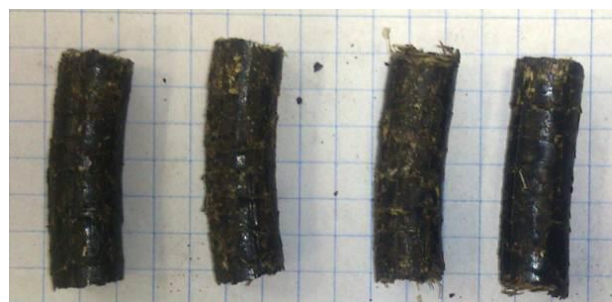
Fig. 7. View of the granulate from a mixture of straw and hard coal with a 15% addition of a potato pulp, obtained at a temperature of 30°C
