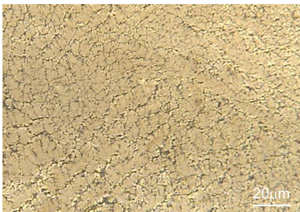
Fig. 3. The microstructure of the melted zone in the surface layer of malleable iron after laser heat treatment. Etched with nitride acid solution
