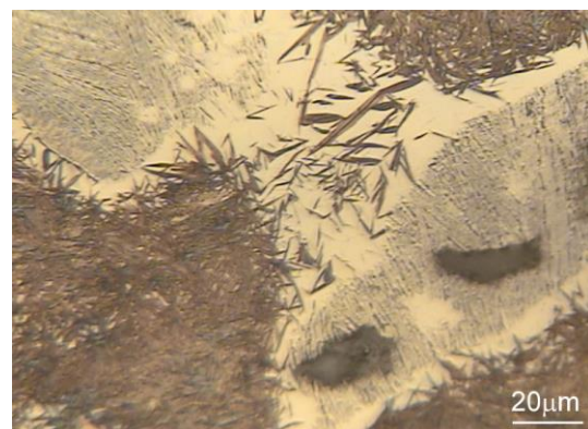
Fig. 5. The microstructure of the transition zone between the melted zone and the hardened zone from the solid state in the surface layer of malleable iron after laser heat treatment. Etched with nitride acid solution
