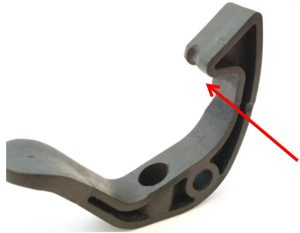
Fig. 2. Traces of wear of the engine cover latch - catch pawl lever [6]
