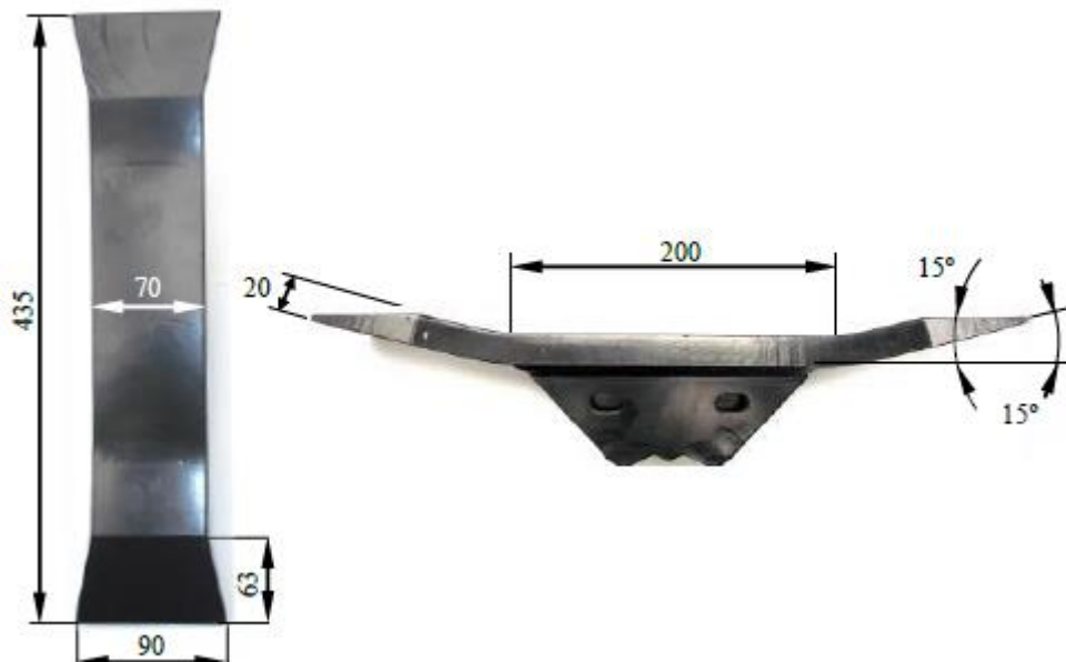
Fig. 1. Main dimensions, shank A (homogeneous material blade)
