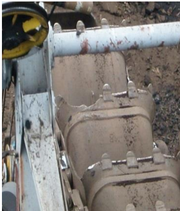
Fig. 5. Damage to the excavator buckets; a) SchRs-900, b) Rs-560, and c) Rs-400 excavators [1] Rys. 5. Uszkodzone czerpaki koparek; a) SchRs-900, b) Rs-560, c) Rs-400 [1]
