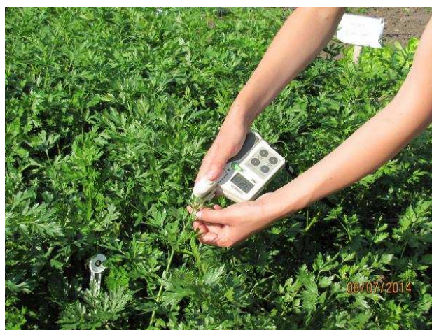
Fig. 2. Measurement of chlorophyll level of parsley leaves with Chlorophyll Meter Minolta Spad 502
