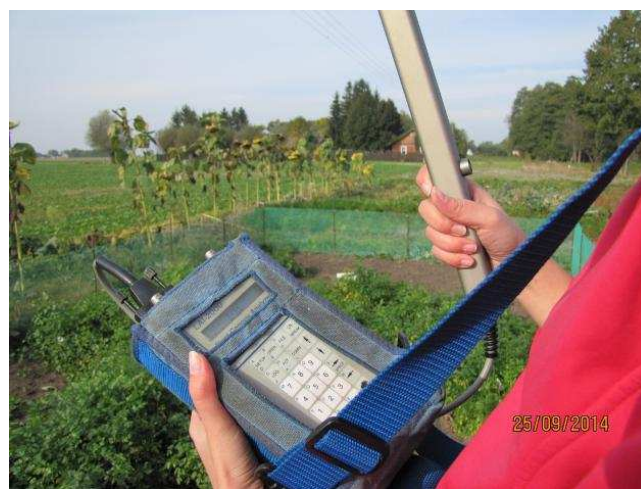
Fig. 3. Measurement of parsley canopy with LAI-2000
