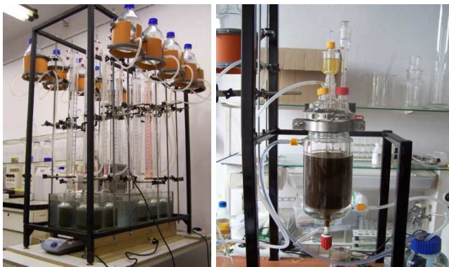
Fig. 3. Research stand for the study of biogas productivity of substrates according to DIN 38414 s.8 (on the left), inoculum station for quasi continuous fermentation work (on the right)
