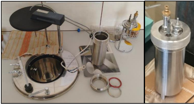
Fig. 3. General view of the position of calorimetric research (left), calorimetric bomb (right)
