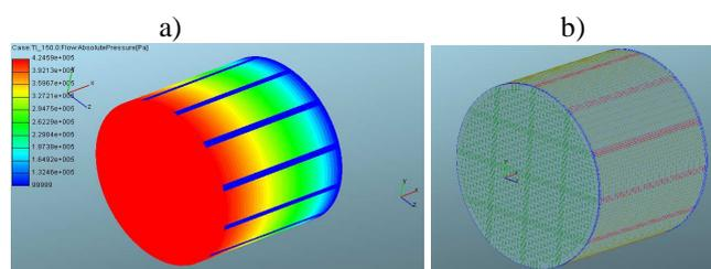
Fig. 6. a) the result of simulation of the absolute flow pressure, b) filter mesh prepared for simulation [7]
