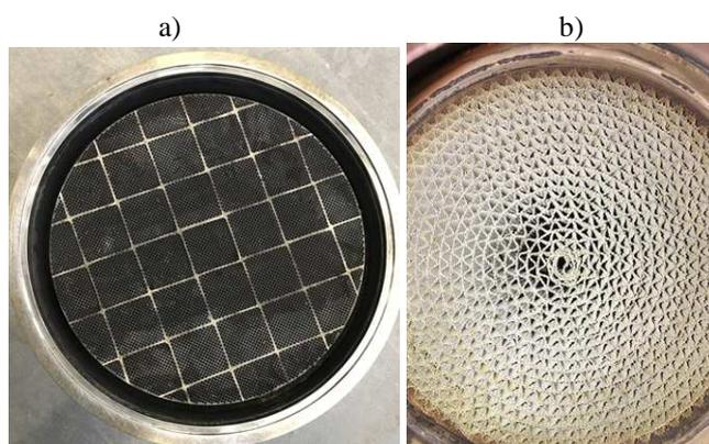
Fig. 7. View of the particulate filter carrier: a) ceramic, b) metal [8]
