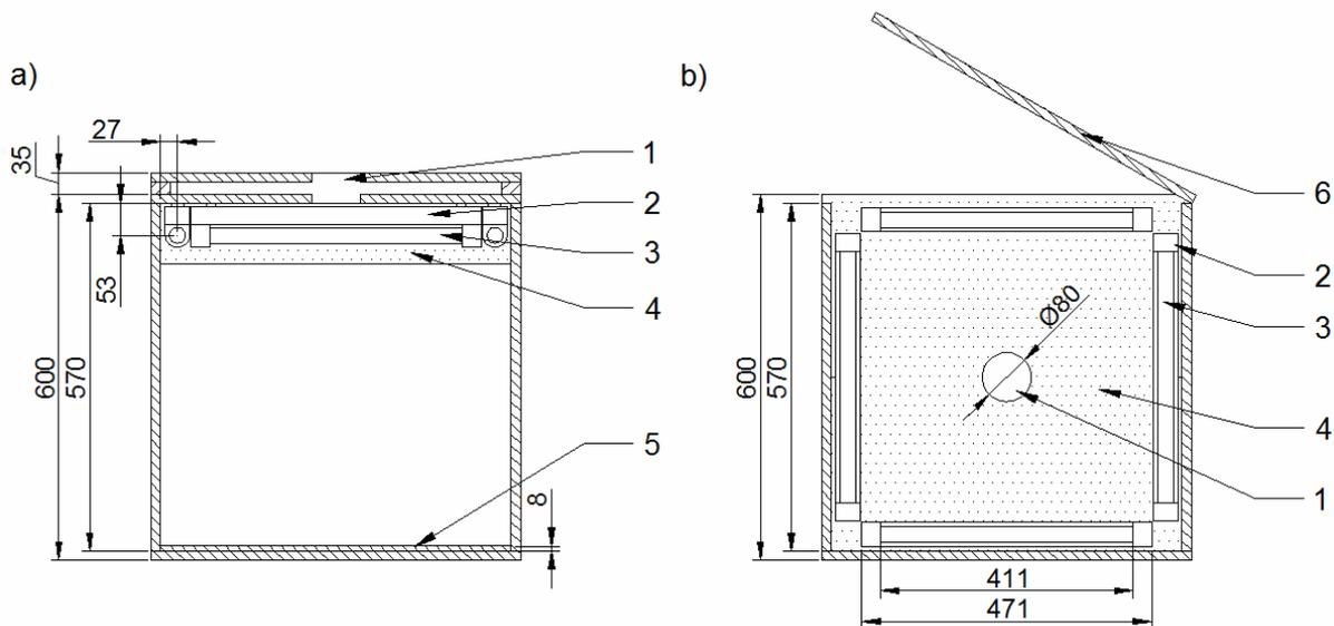
Fig. 1. Technical drawing of photographic chamber (dimensions in millimeters): a – the inside of chamber viewed from the side, b – the view of the upper inner surface of chamber, 1 – the hole for a camera lens, 2 – fluorescent lamp fixture, 3 – fluorescent lamp, 4 – reflective foil, 5 – removable tray for composted material, 6 – opening front plate [10]
