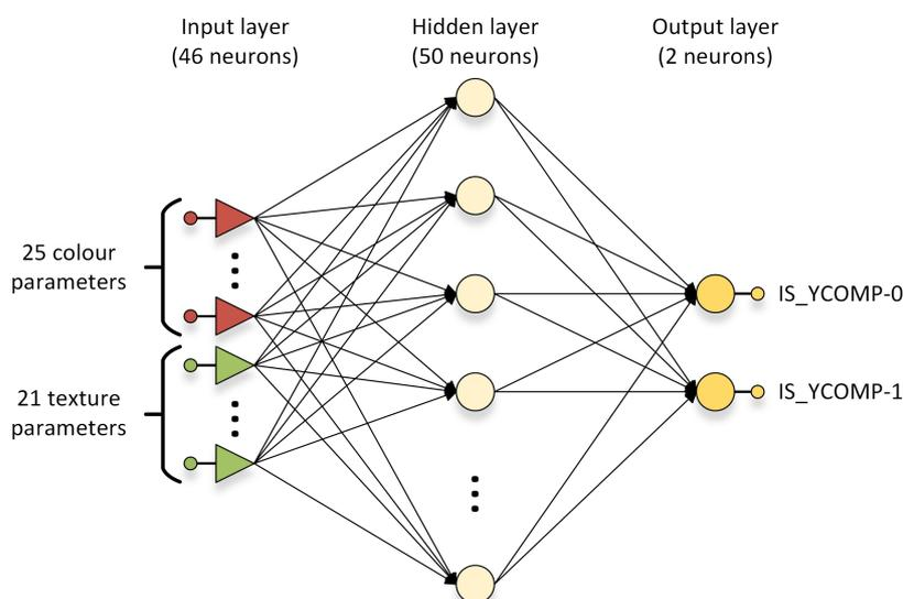
Fig. 3. The initial structure of neural networks [8]
