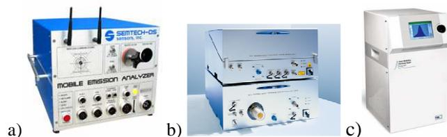
Fig. 8. Pictures of the exhaust measurement devices used: a) SEMTECH DS., b) AVL MSS, c) TSI 3090 EEPS [10, 11, 12]
