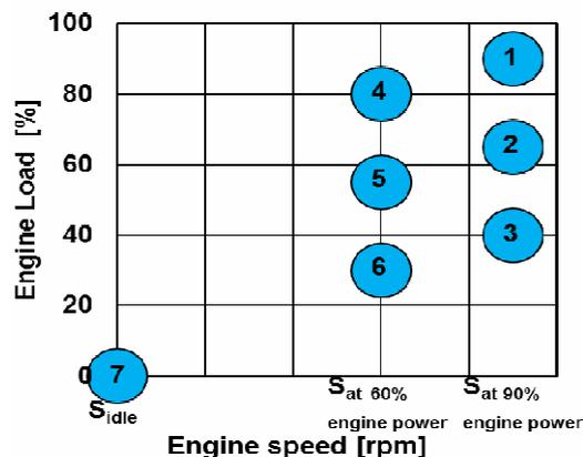
Fig. 7. The NRSC test points after modification [9]
