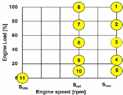
Fig. 4. The NRSC test measurement points [9]
