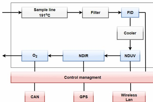
Fig. 9. SEMTECH DS operation schema [10]
