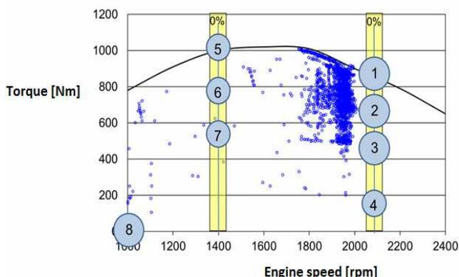
Fig. 6. Comparison of agricultural tractor engine operating range in real conditions with NRSC test points [9]
