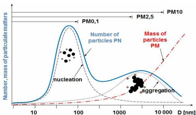
Fig. 2. The idealized relation between the size of particles and their number and mass for exhaust gases from the CI engine [8]
