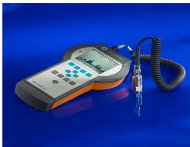
Fig. 5. Accelerometer with a Vibrotest Shenck 60 reader [7]
