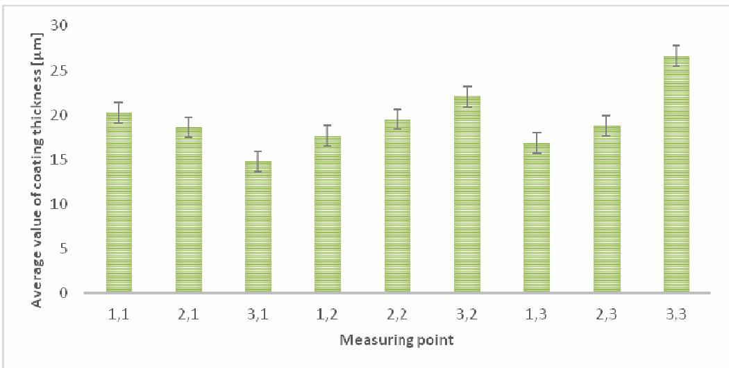
Fig. 5. Distribution of the average thickness of the coating applied by a spray after testing in a salt spray chamber [3]
