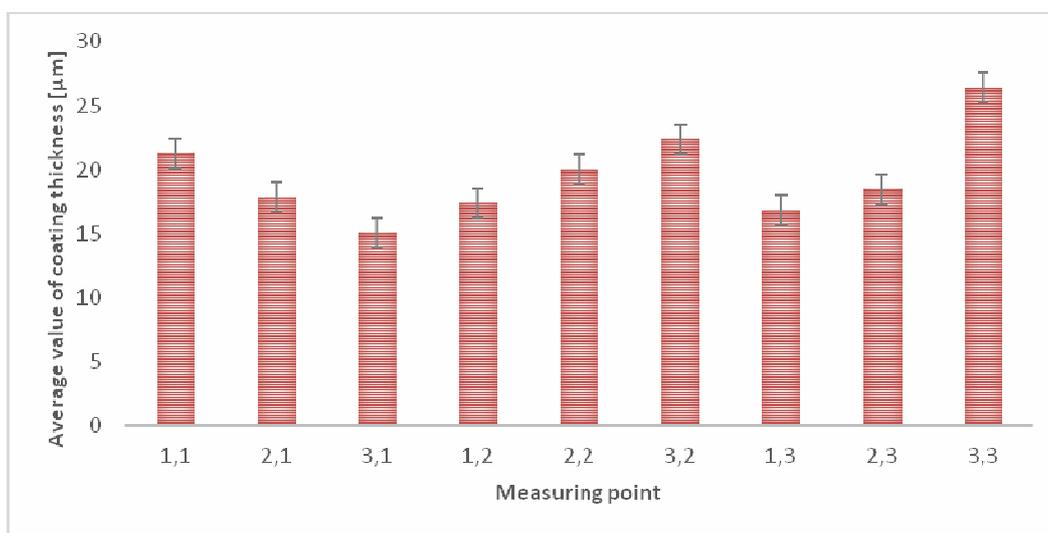
Fig. 4. Distribution of the average thickness of the coating applied by a spray before testing in a salt spray chamber [3]
