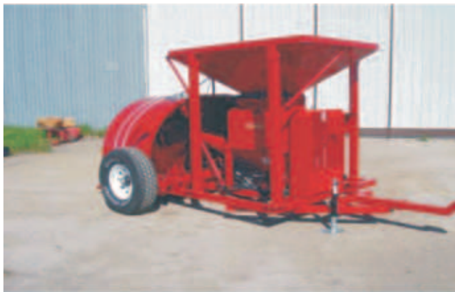
Rys. 7. Prasa silosująca z zespołem do rozdrabniania ziarna (prod. New Concept Industries Ltd.) Fig. 7. Silage compactor equipped with grain crushing unit (manufactured by New Concept Industries Ltd.)
