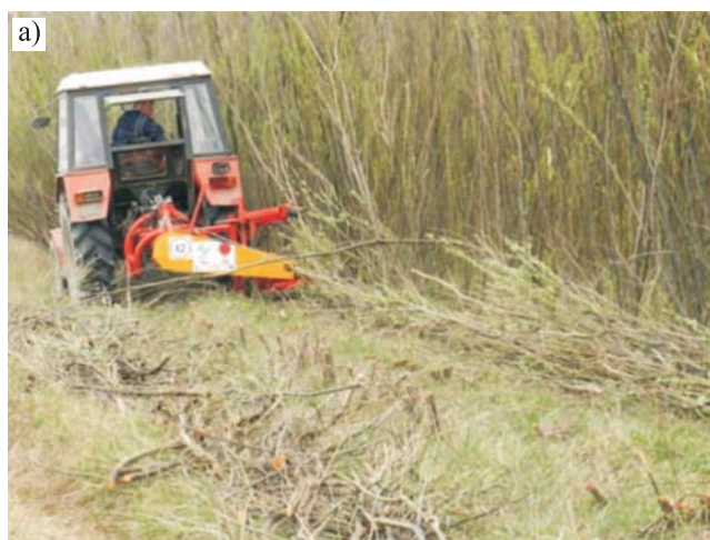
Fig. 2. Harvester cutting unit: 1 - saw drive belt transmission, 2 - arm of saw suspension, 3 - handle to change the position of the arm of saw suspension from transport to work and vice versa, 4 - saw blade, 5 - blade guard with vertical guidance element, 6 - the red guiding cut stems on the screw feeder
