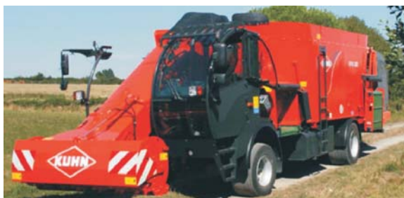
Rys. 4. Samojezdny wóz paszowy SPW Compact firmy KUHN [1] Fig. 4. A self-propelled SPV Compact fodder carriage of KUHN [1]
