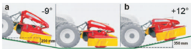
Rys. 4. Kosiarka NOVOCAT z systemem alpha motion Fig. 4. Mower NOVOCAT with alpha motion system
