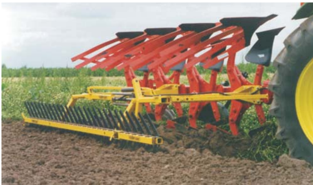
Rys. 11. Listwa nożowa (Kerner) zintegrowana z plugiem [11] Fig. 11. Cutterbar (Kerner) integrated with the plough [11]
