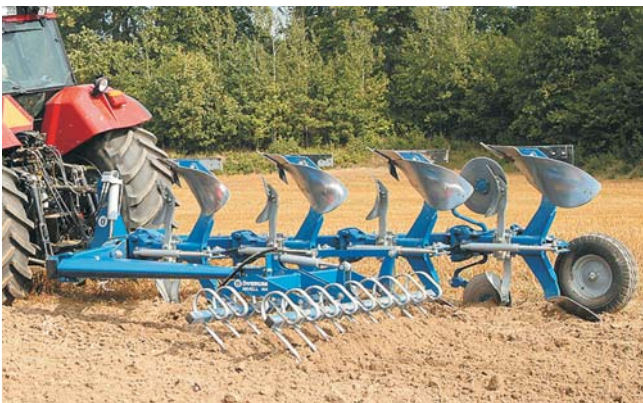
Rys. 12. Brona Nivell (Overum) zintegrowana z plugiem [12] Fig. 12. Nivell harrow (Overum) integrated with the plough [12]
