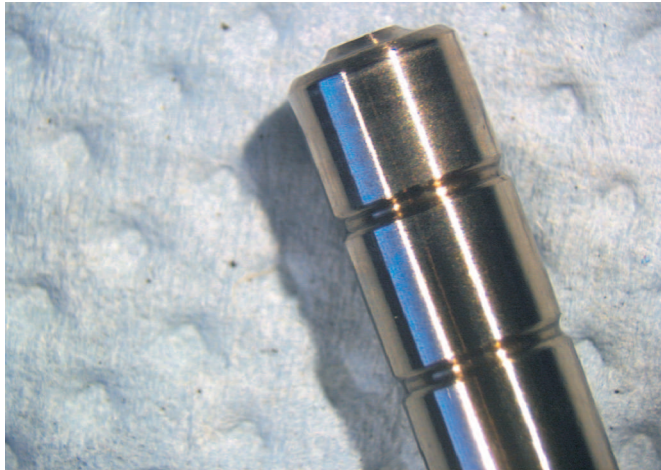
Fig. 18. Needle valve of the nozzle CR BOSCH; visible yellowish deposit resulting from biofuels' use and effect of organic acids contained in fuel
