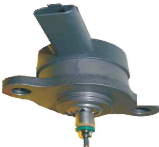
Rys. 9. Regulator ciśnienia pompy z uszkodzonym tensometrem pomiarowym Fig. 9. Pressure regulator of the pump with damaged measuring strain gauge
