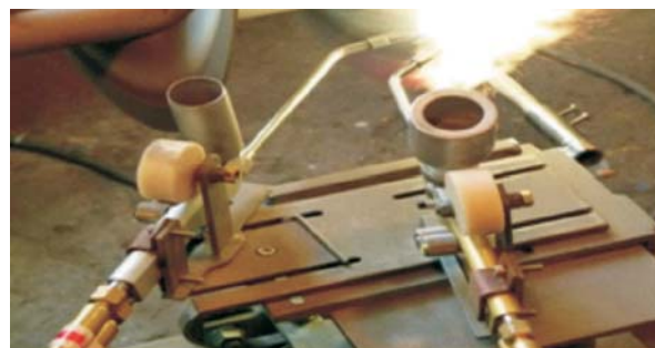
Fig. 3. Regeneration by metal spraying method of Cardan shaft
