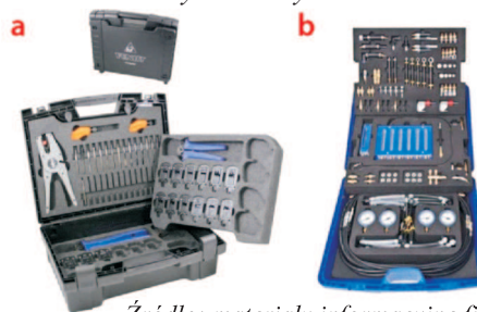
Fig. 10. Fendt tractor diagnostic equipment: a) flow-meters for flow testing in the hydraulic system, b) digital flow measurement kit in the hydraulic system
