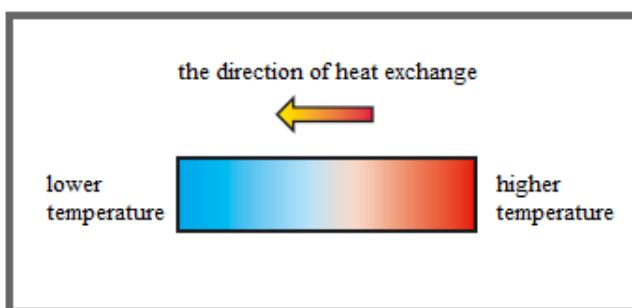
Fig. 1. Graphic example of heat conduction [3]
