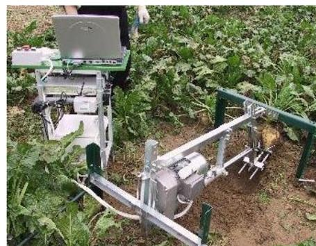
Fig. 3. Stand for measuring the horizontal component of the force acting on the lifter share [4]
