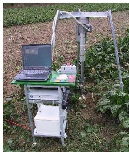
Fig. 4. Stand for measuring the vertical component of the force acting on the lifter share [4]
